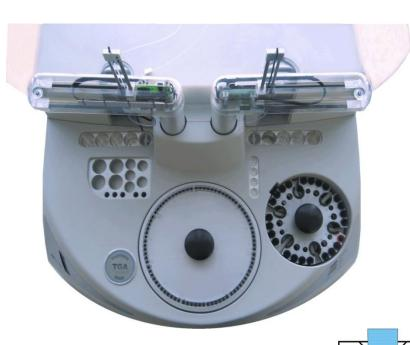
For thrombin generation measurement 4 channels with special fluorometric TGA modules consisting of an UV LED (365nm) for excitation and a photodiode for measurement of the emitted signal.
